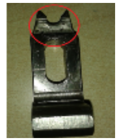
Clamping pad wear out
